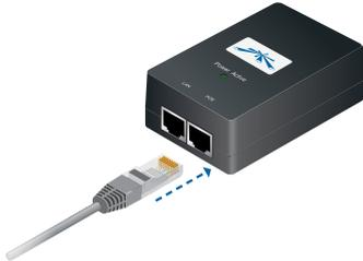
2. Connect an Ethernet cable from your LAN to the Ethernet port labeled **LAN** on the *PoE GigE Adapter*.
